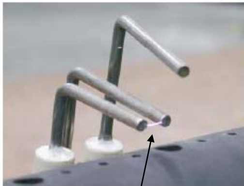
Correct positioning: A spark is generated at the Spark point.
